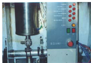
Fig.3 The PM actuator(left) and its control unit(right) for the 12kV indoor vacuum circuit breaker
